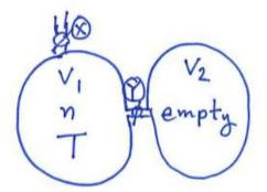
Initially, the right flask is completely empty while the left flask contains n moles of ideal gas at temperature T. Both stopcocks  $\mathbf{X}$  and  $\mathbf{Y}$  are closed. Stopcock  $\mathbf{Y}$  is then opened and gas effuses from one flask to the other. It initially effuses an amount  $a_{first}$  in a small unit of time.
